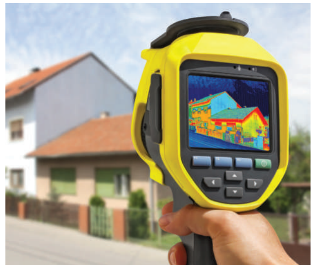
Infrared thermal vision image showing lack of thermal insulation on house or without facade insulation.
